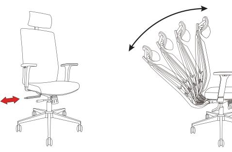
Rotate the knob to increases or reduces the tightness of chair back reclining.
