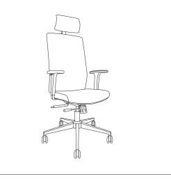
The angle and height of headrest is adjustable. Lift the handle to adjust chair height. Lift the armrest button, the armrest can be Rotate the PU arm pad to adjust the angle. The PU arm pad can be moved forward and backward. adjusted up and down.
