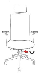
Lift the handle, the seat cushion can be adjusted forward and backward.
